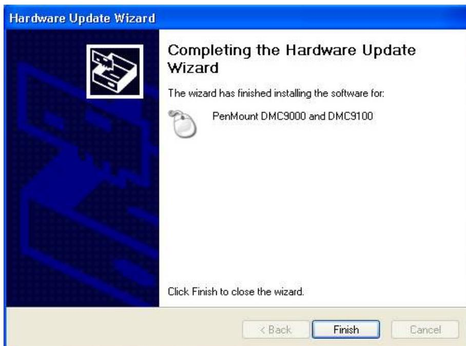
7. The screen will show "PenMount DMC9000 and DMC9100" under "Mice and other pointing devices" as below if your installation is successful. Otherwise, you need to go back to the 1 to 6 to reinstall the driver again.
