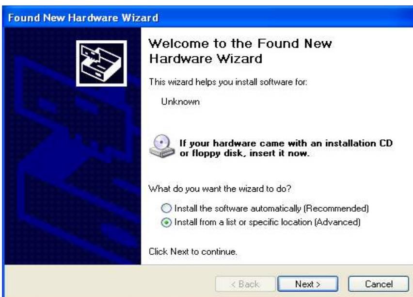
2. If your screens' message does not show as Fig. 1 , then from “Start”, select “Control Panel”, select “System”, select “Hardware”, select “Device Manager”, then double click the “Unknown device
